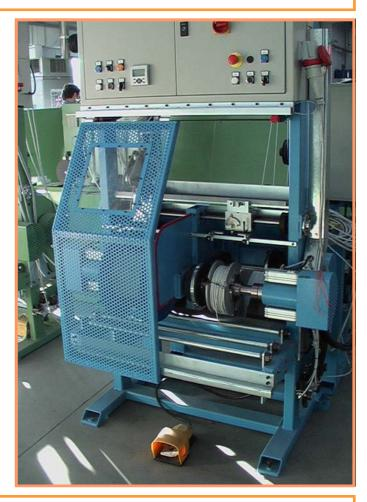
The take up type "AV 2X400 CA 300" allows the packaging of bobbins or coils with dimension up to Ø 400 X 200 mm for bobbins and Ø 400 X 90 mm for coils.
